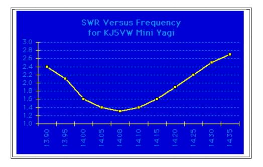
I was pleasantly surprised to see that the bandwidth between the SWR 2.0 points was more than 200 Khz. I had expected a much narrower bandwidth because of the wire elements and the inductive loading coils.
